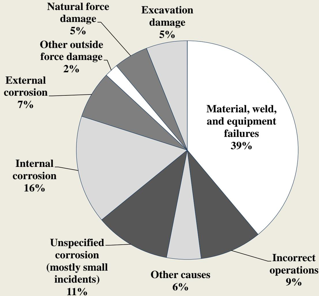
**Causes of crude oil pipeline releases reported to PHMSA, 2002 to 2011**
